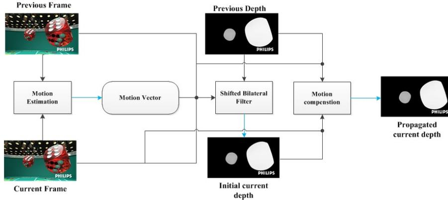
Figure 2. Depth propagation
